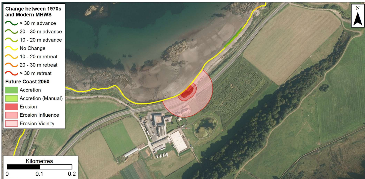
Figure 6.36: Possible future coastline position in 2050 based on rates between 1970 and Modern MHWs data at Woodland Bay. Getmapping are our current providers of Scotland-wide digital aerial imagery© Getmapping plc.
