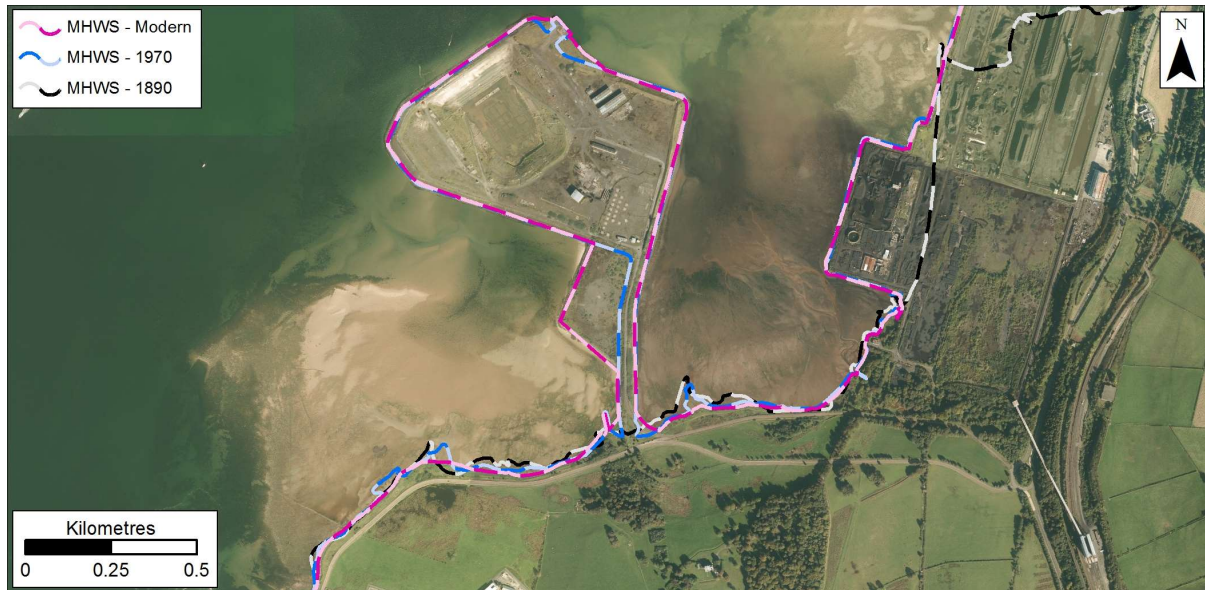
Figure 6.27: MHWS position in 1890, 1970s, and Modern datasets at Hunterston B Nuclear Power Station. Getmapping are our current providers of Scotland-wide digital aerial imagery© Getmapping plc.
