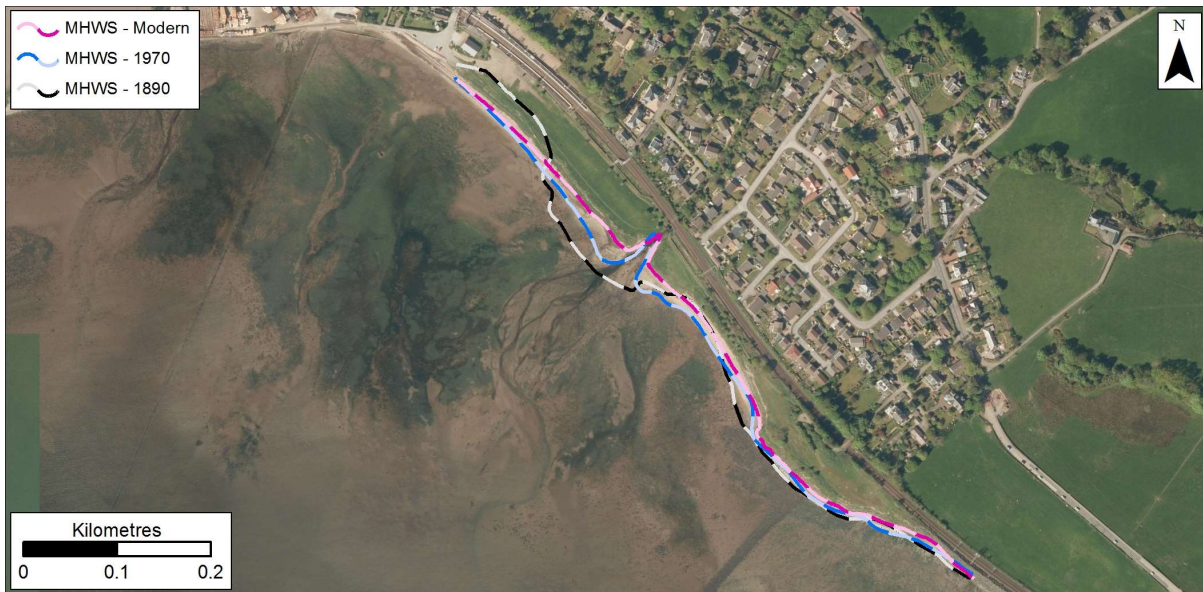
Figure 6.23: MHWS position in 1890, 1970s, and Modern datasets at Cardross. Getmapping are our current providers of Scotland-wide digital aerial imagery© Getmapping plc.
