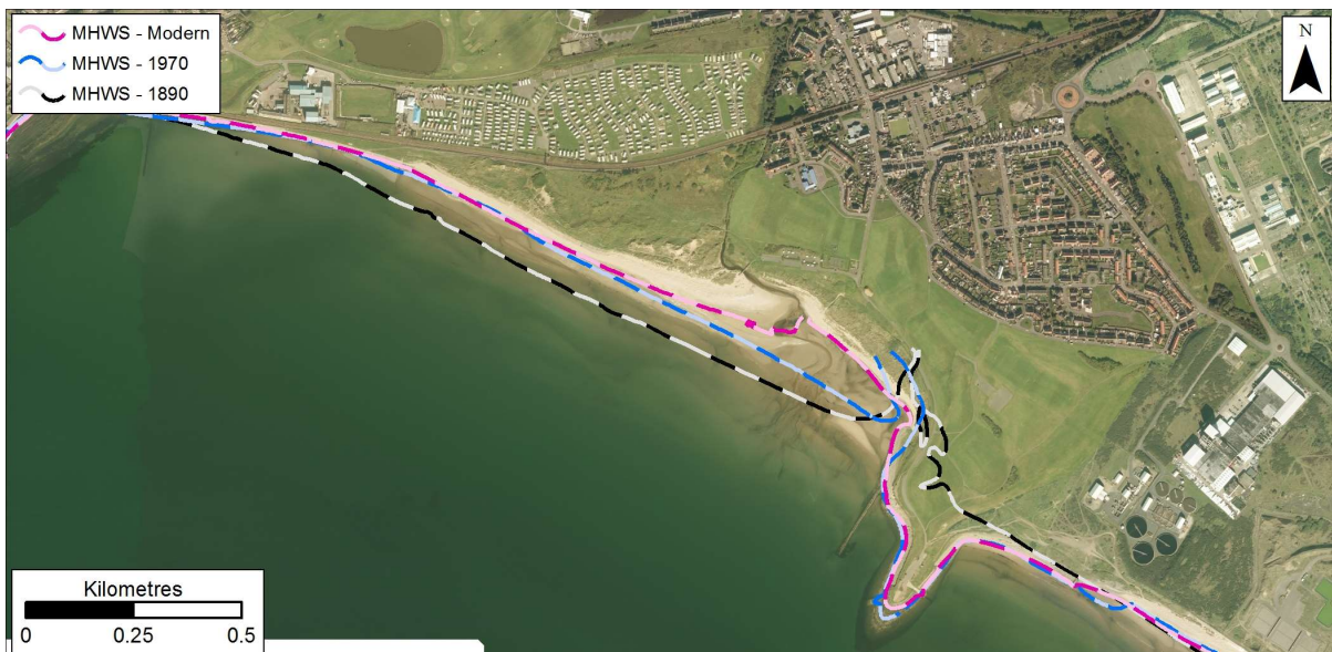
Figure 6.31: MHWS position in 1890, 1970s, and Modern datasets at Saltcoats. Getmapping are our current providers of Scotland-wide digital aerial imagery© Getmapping plc.
