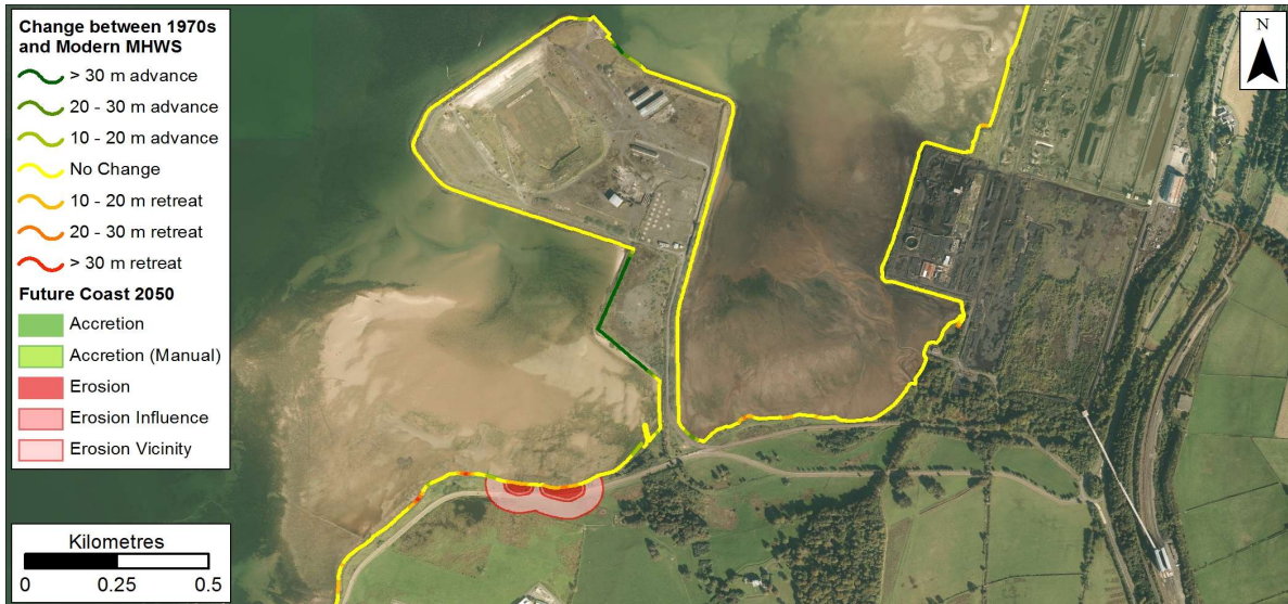
Figure 6.28: Possible future coastline position in 2050 based on rates between 1970 and Modern MHWS data at Hunterston B Nuclear Power Station. Getmapping are our current providers of Scotland-wide digital aerial imagery© Getmapping plc.
