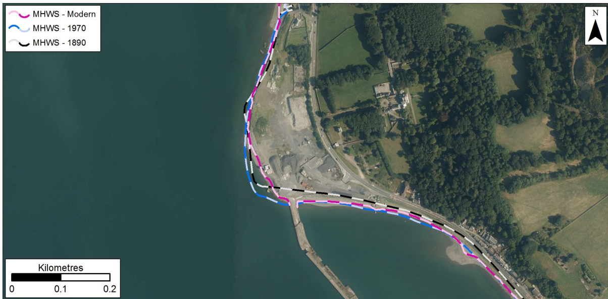
Figure 6.39: MHW position in 1890, 1970s, and Modern datasets at Cairnryan Old Pier. Getmapping are our current providers of Scotland-wide digital aerial imagery© Getmapping plc.
