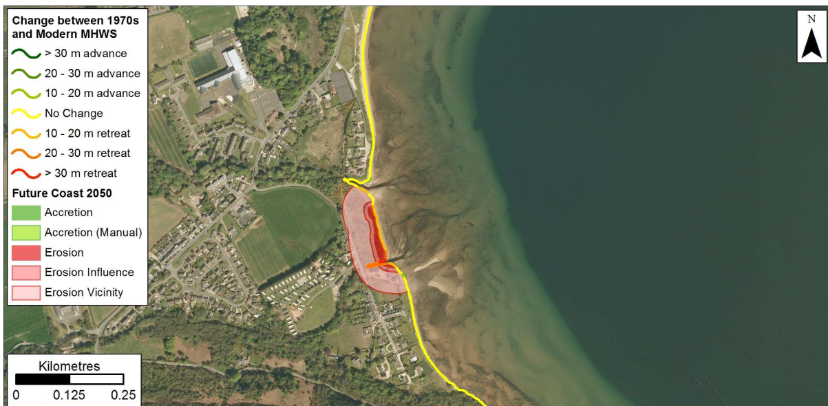
Figure 6.11: Possible future coastline position in 2050 based on rates between 1970 and Modern MHWS data at Lamlash. Getmapping are our current providers of Scotland-wide digital aerial imagery© Getmapping plc.
